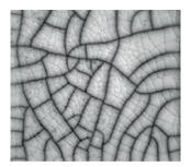
The spider-web pattern of cracking is different from a break in the aspect that it cannot be felt on the surface, unless using a fingernail; however, it does become more visually apparent when the surface is dusty or magnified. While these may appear as imperfections, 'crazing' does not affect the performance or life span of your ceramic charcoal barbecue; therefore, not a warranty issue. The process of 'crazing' effectively increases the toughness of the unit.
